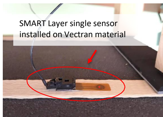
Figure 2: Sensors installed on Vectran material
