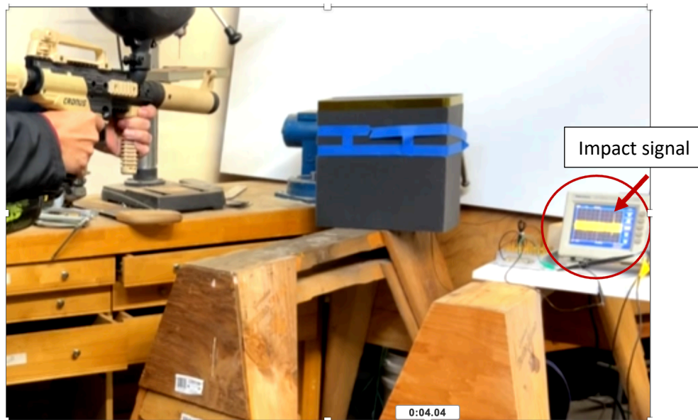
Figure 8: Impact test setup using a paintball gun for impacts
