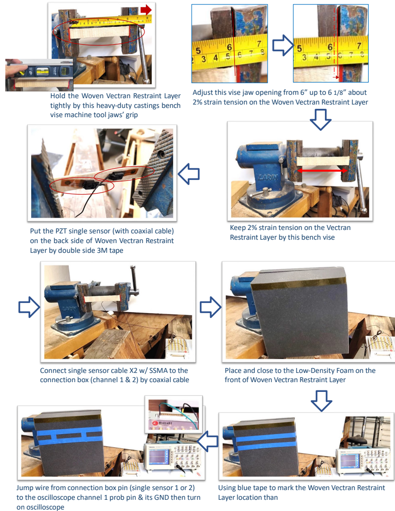
Figure 7: Test setup using 2% strain
