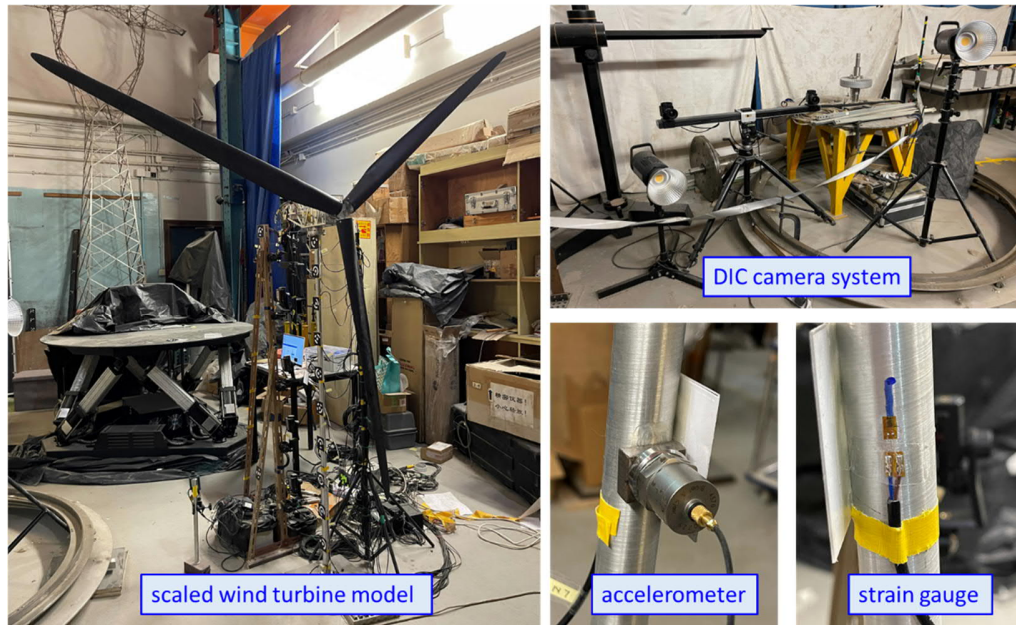
Figure. 2. The scaled WT model and SHM sensing system
