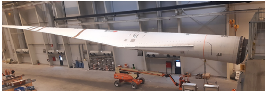
Figure 1. Wind turbine blade mounted on test stand at Siemens Gamesa Blade Test Center in Aalborg, Denmark.
