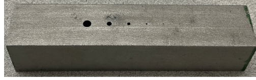
Figure 1. Actual steel sample with a dimension of 154.2 mm \times 32 mm. It has six holes with varying diameters at the center horizontal line. All numerical models were built on this steel sample.
