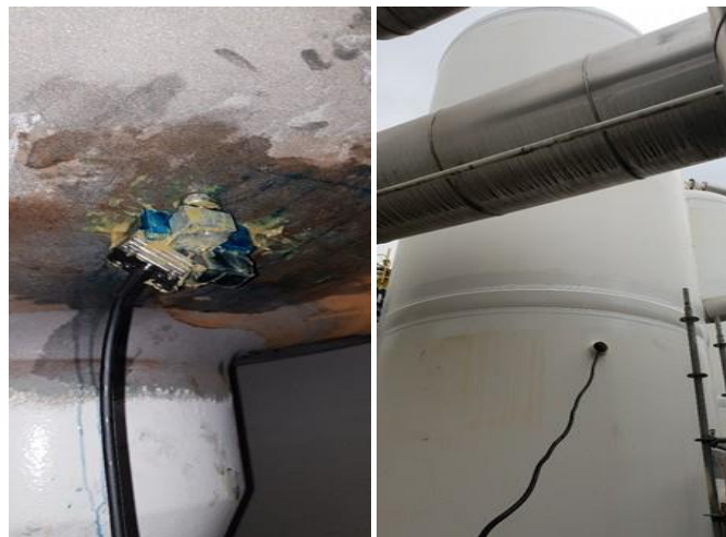
Figure 4: Connected probe, fixed to the bottom head (left), into the skirt volume (right).
