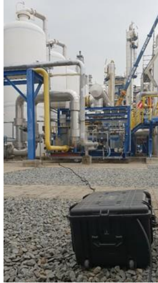
Figure 5: UT and electronic system to pilot the connected probe at Air Liquide site.
