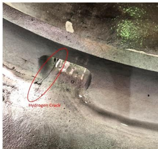
Figure 3. Fatigue crack at the support/head weld location.
