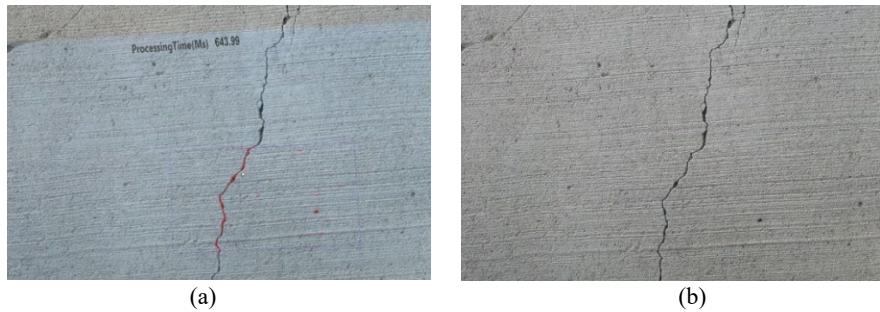
Figure 2: crack detection with AR-HMD devices; (a) unprocessed image (b) processed image inside the AR-HMD device
