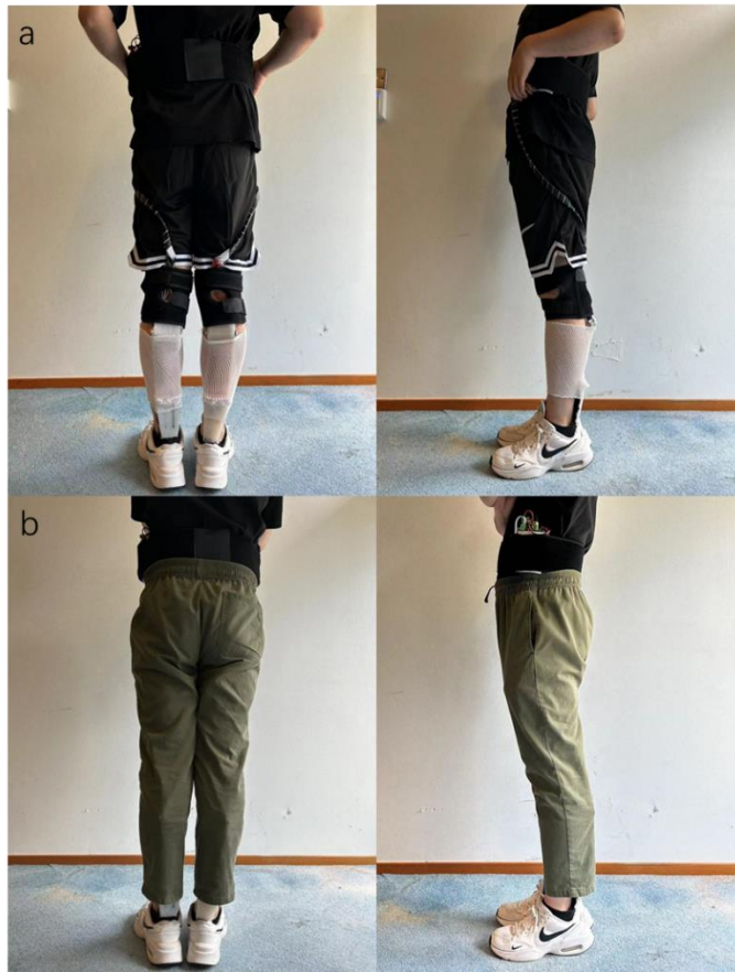
Figure 2. Wearable gastrocnemius lateralis (GL) muscle-mimetic robot. a. subjects wore short pants and robots and b. robots wear underneath long pants.
