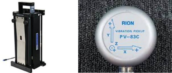
Figure 4. Equipments (left: Shaker, right: Accelerometer)
