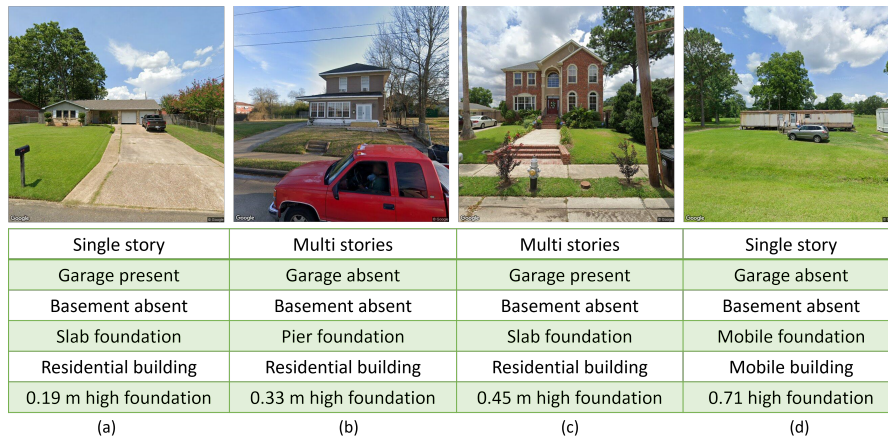
Figure 2. Sample predictions of heterogeneous data fusion. All the classification attributes are predicted correctly. The actual foundation heights are (a) 0.1524 m, (b) 0.4572 m, (c) 0.4572 m, and (d) 0.762 m, which are reasonably close to the estimated heights.
