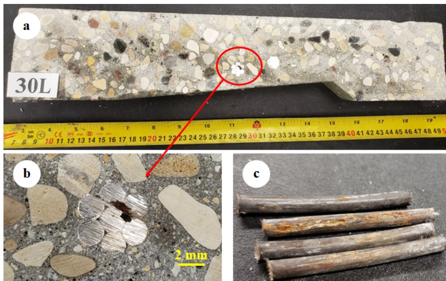
Figure 7. The right side of the 30th slice (a), Visual signs of corrosion on the cross-section of tendon 1 on the left side of the 30th slice (b), and corroded wires of tendon 1 from the 30th slice (c).
