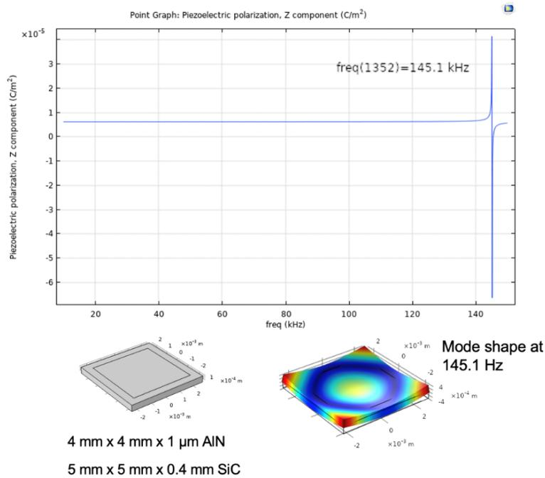
Figure 1. Sensor dimension and frequency response
