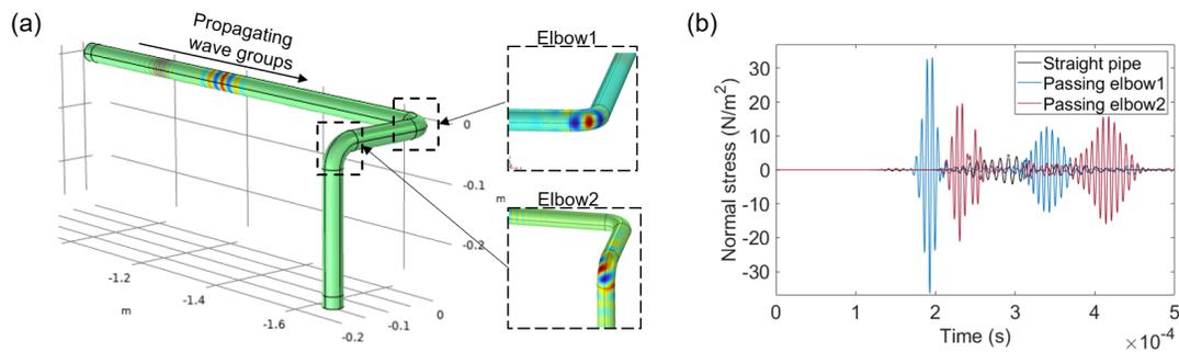
Figure 5. Influence of elbows on wave propagation, (a) wave propagating on the straight pipe and wave focusing when passing the elbow1 and elbow2; (b) comparison of time domain signals with respect to the influence of the existence of elbows.
