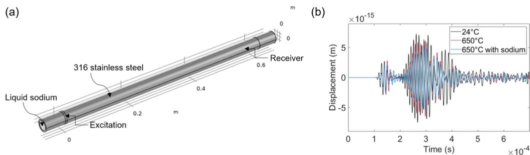
Figure 4. Influence of temperature and liquid sodium on wave propagation, (a) numerical models, and waveforms received 0.6 m away from the excitation, (a) hollow pipe at 24°C (b) hollow pipe at 650°C (c) pipe filled with liquid sodium at 650°C.
