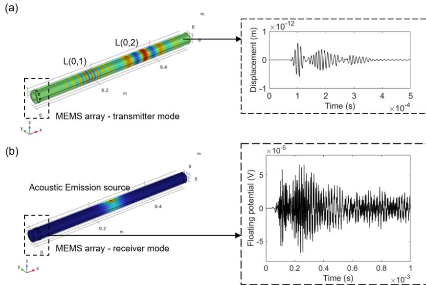
Figure 3. The dual functionality of MEMS array (a) the generation of pure Lamb wave modes with eight circular sensors positioned around the pipe circumference, (b) the simulation of acoustic emission signal, and acoustic emission signal detected by the MEMS array.
