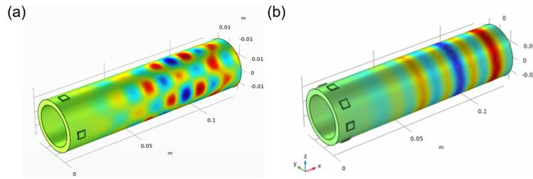
Figure 2. Numerical models determine the number of sensors at the pipe circumference to generate plane waves, (a) four sensors and (b) eight sensors.
