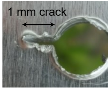
Figure 8. Photograph of the 1 mm long crack created on the aluminium sample.
