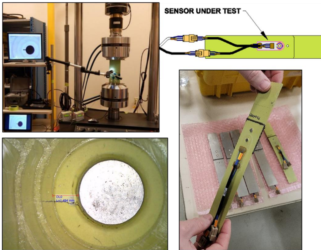
Figure 4. Fatigue testing to assess CVM performance in 737 Aft Pressure Bulkhead application.
