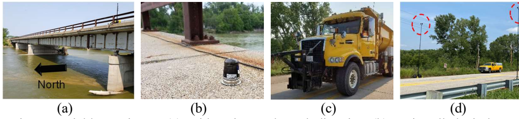
Figure 5. Field experiment: (a) Bridge view and North direction, (b) An installed wireless accelerometer, (c) A tri-axial dump truck, and (d) Installed traffic cameras.
