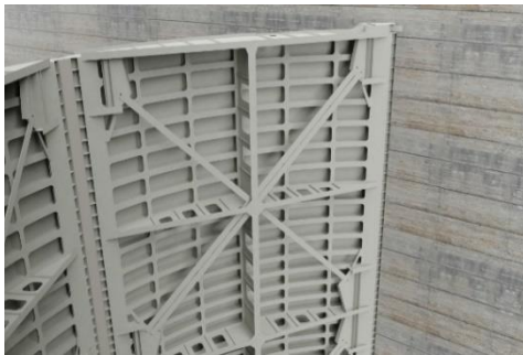
Figure 2. Undeformed PBGM miter gate
