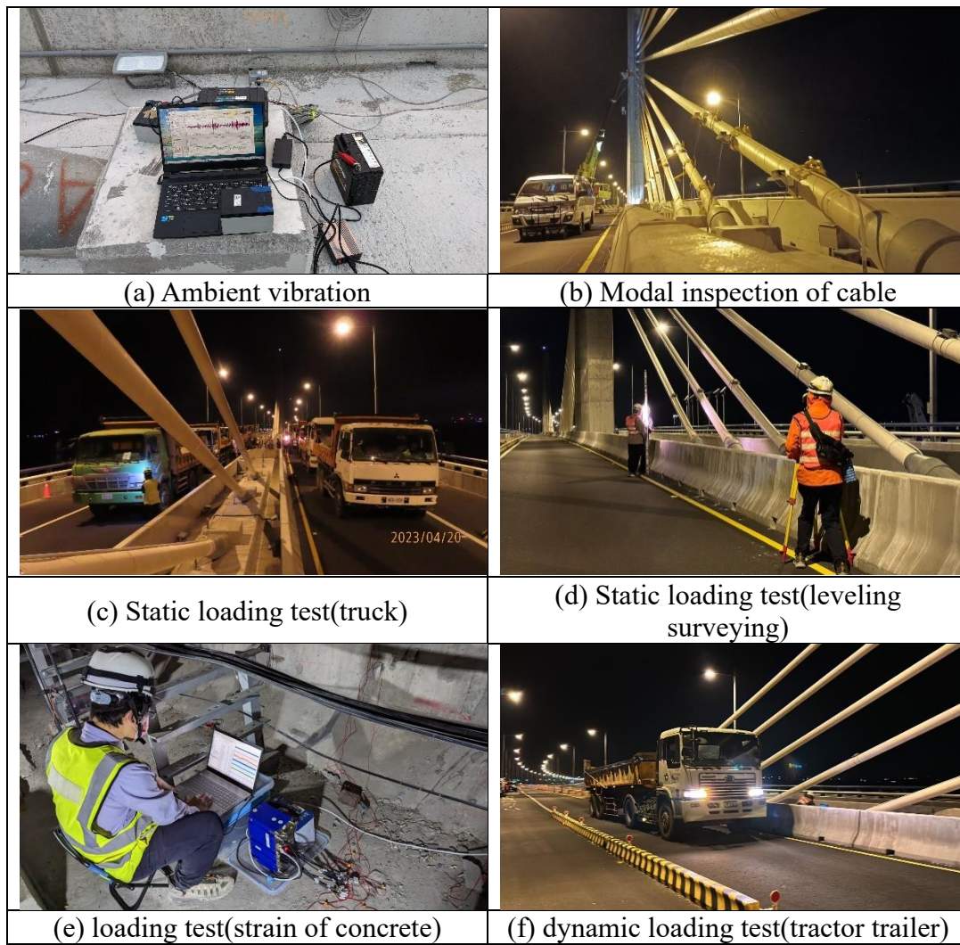
Figure 3. In-situ testing of Kinmen bridge
